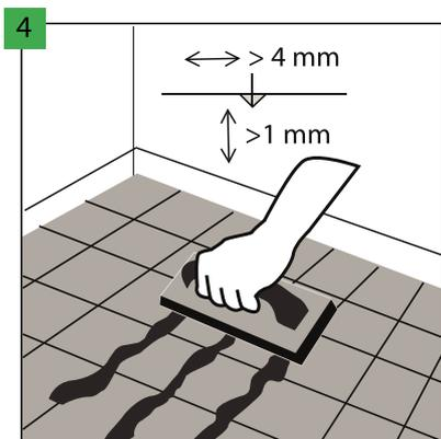
In the case of installation on the substrate covered with ceramic tiles, fill the tile joints with the gap wider than 4 mm and deeper than 1 mm with a durable compound for the filling of points, e.g. resin grout. Installation is allowed on tiles with grouts not wider than 5 mm and 1 mm deep without using levelling compound, provided the Multiprotect Hardlay or Vinclic Solid are used as underlay.
