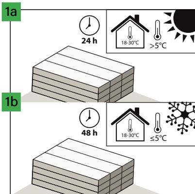
If the temperature is  $>5^{\circ}\text{C}$  during transport, the acclimatization time in a room with a temperature of  $18-30^{\circ}\text{C}$  should be min. 24 hours (in the premises where they will be installed). However, in case of temperature  $\leq 5^{\circ}\text{C}$  during transport, acclimatization time in a room with a temperature of  $18-30^{\circ}\text{C}$  should be min. 48 hours.
